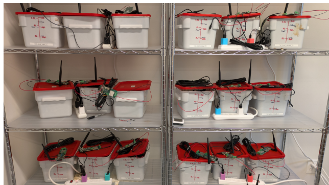
(a) ENTS monitoring 18 SMFCs to characterize open vs closed circuit behaviors
