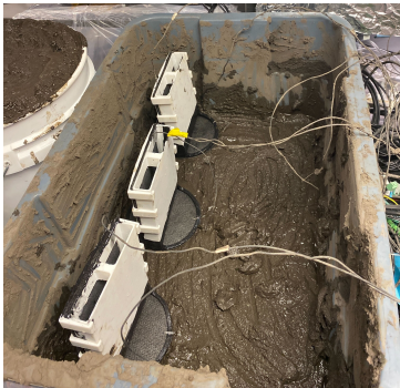
(a) Step 3 of the procedure from Installing SMFCs . The cells are spaced apart to ensure they are not touching, and there is about 5 cm of soil underneath the anodes.
