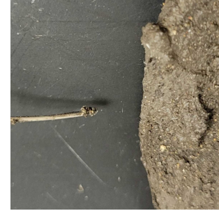
(b) Dirty/disconnected wire.
